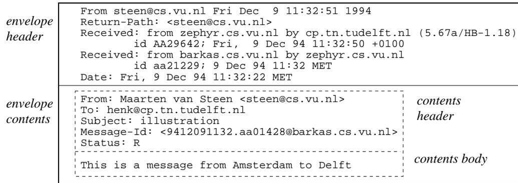
**Figure 10.10** An example of the structure of an envelope sent via electronic mail.
