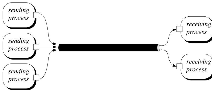
**Figure 6.12** The principle of a channel in message-based communication.
