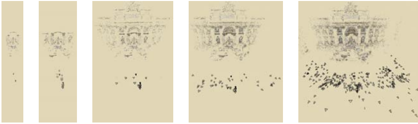
Figure 7.11 Incremental structure from motion (Snavely, Seitz, and Szeliski 2006) © 2006 ACM: Starting with an initial two-frame reconstruction of Trevi Fountain, batches of images are added using pose estimation, and their positions (along with the 3D model) are refined using bundle adjustment.
