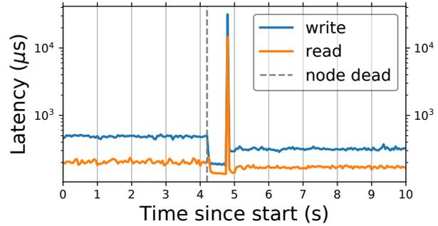
(a) A timeline for GCS read and write latencies as viewed from a client submitting tasks. The chain starts with 2 replicas. We manually trigger reconfiguration as follows. At  $t \approx 4.2s$ , a chain member is killed; immediately after, a new chain member joins, initiates state transfer, and restores the chain to 2-way replication. The maximum client-observed latency is under 30ms despite reconfigurations.
