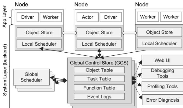
Figure 5: Ray’s architecture consists of two parts: an *application* layer and a *system* layer. The application layer implements the API and the computation model described in Section 3, the system layer implements task scheduling and data management to satisfy the performance and fault-tolerance requirements.
