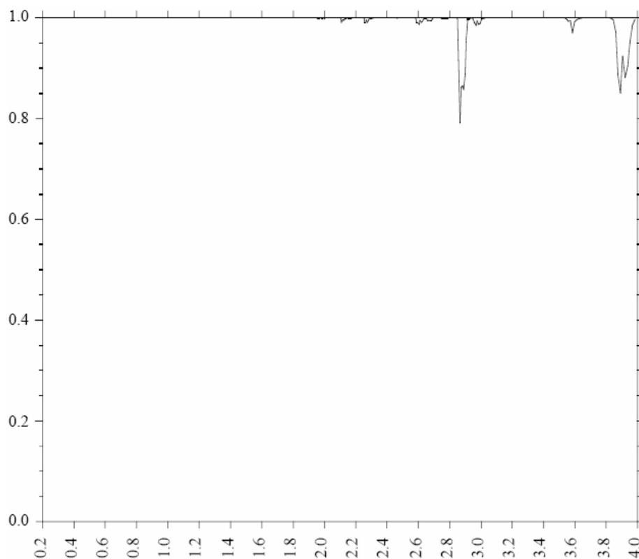
**Fig. I-5.** Spectral transmittance of N<sub>2</sub>O.
