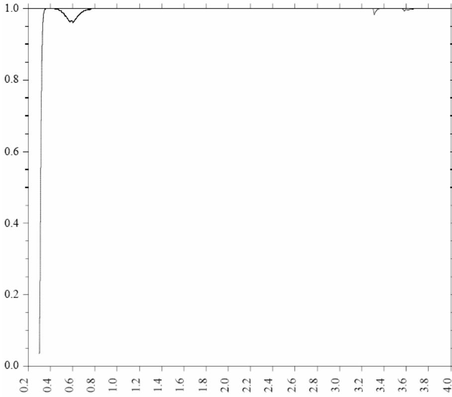
**Fig. I-2.** Spectral transmittance of O<sub>3</sub>.
