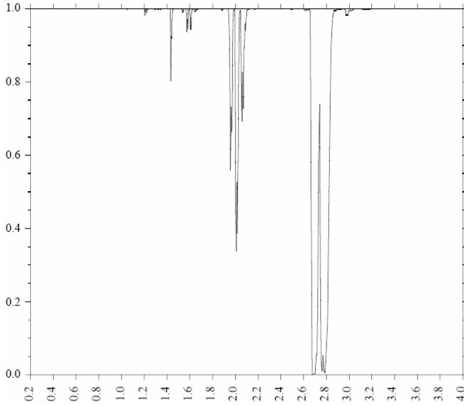
**Fig. I-3.** Spectral transmittance of CO<sub>2</sub>.
