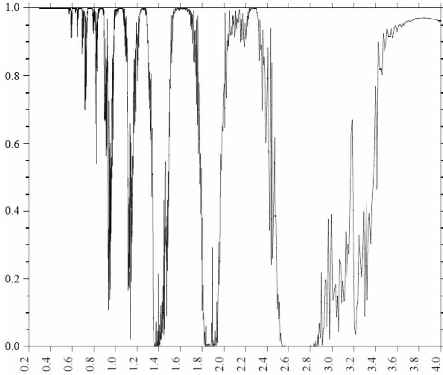
**Fig. I-1.** Spectral transmittance of H<sub>2</sub>O.
