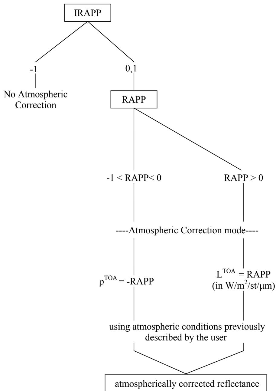
Fig. A-9. Detailed flow chart for atmospheric correction mode.
