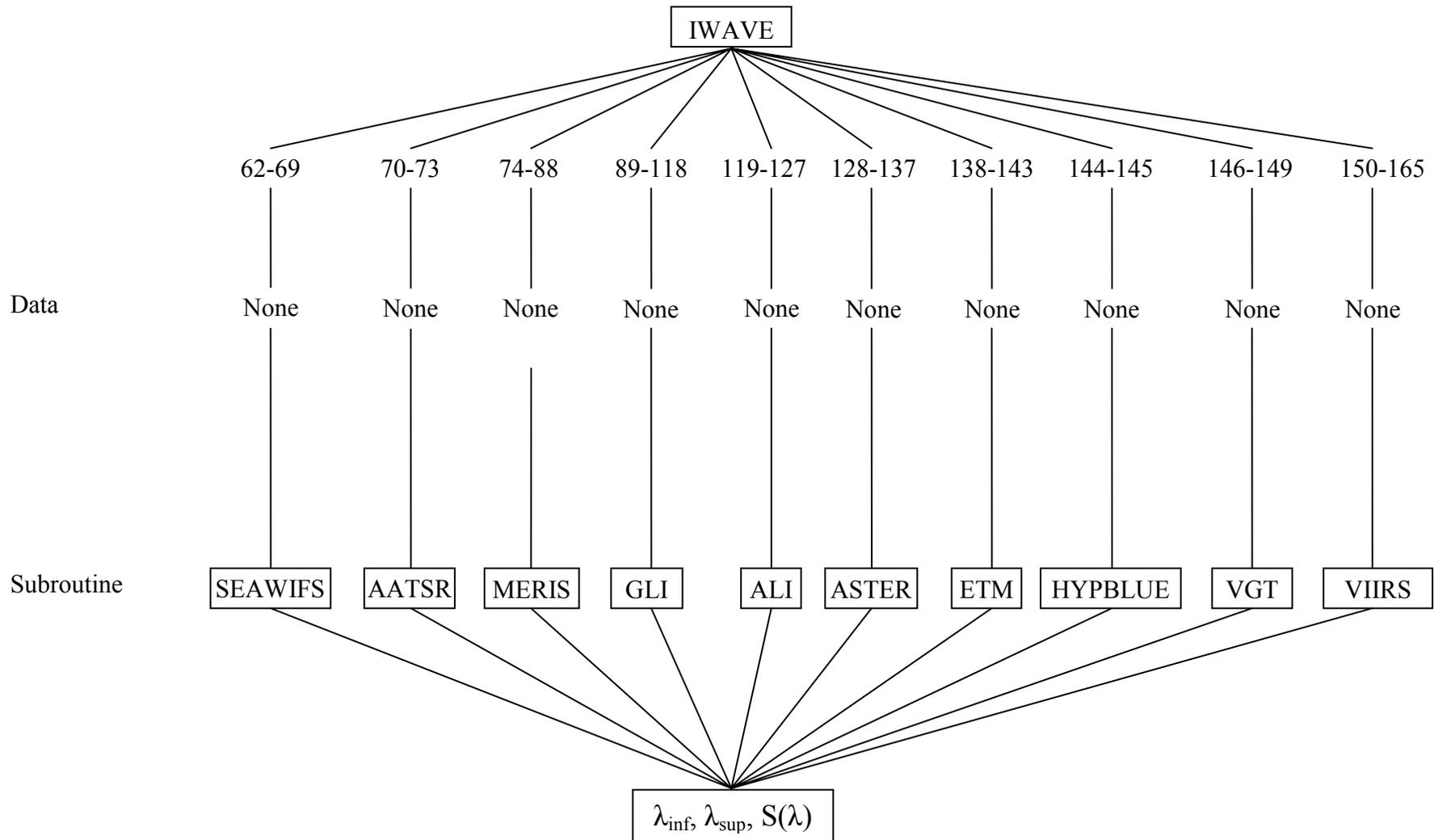
Fig. A-7'. Detailed flow chart (Part II) for spectral band definition of extreme wavelengths and filter function
