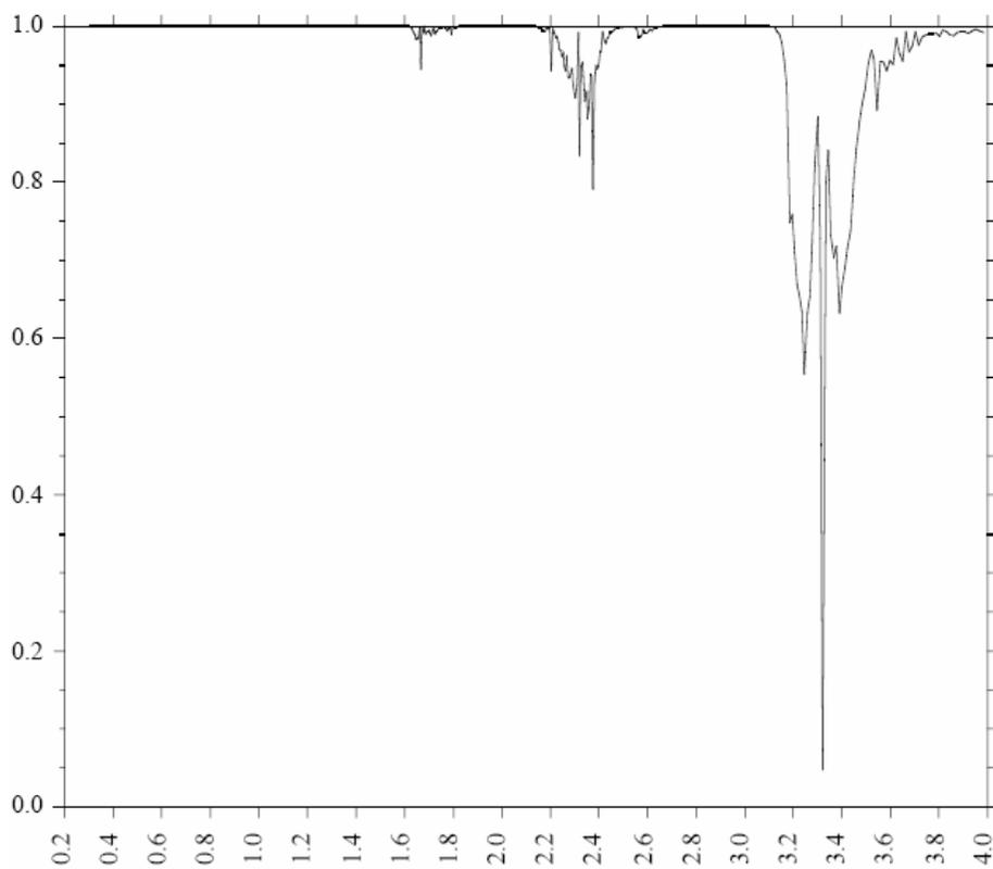
**Fig. I-6.** Spectral transmittance of CH<sub>4</sub>.
