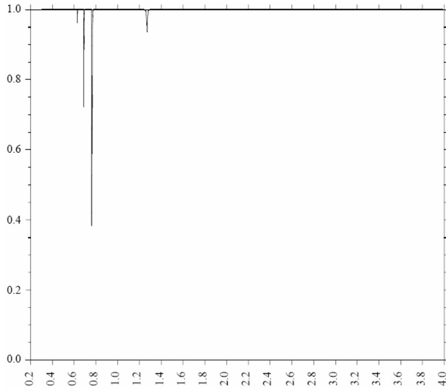
**Fig. I-4.** Spectral transmittance of O<sub>2</sub>.
