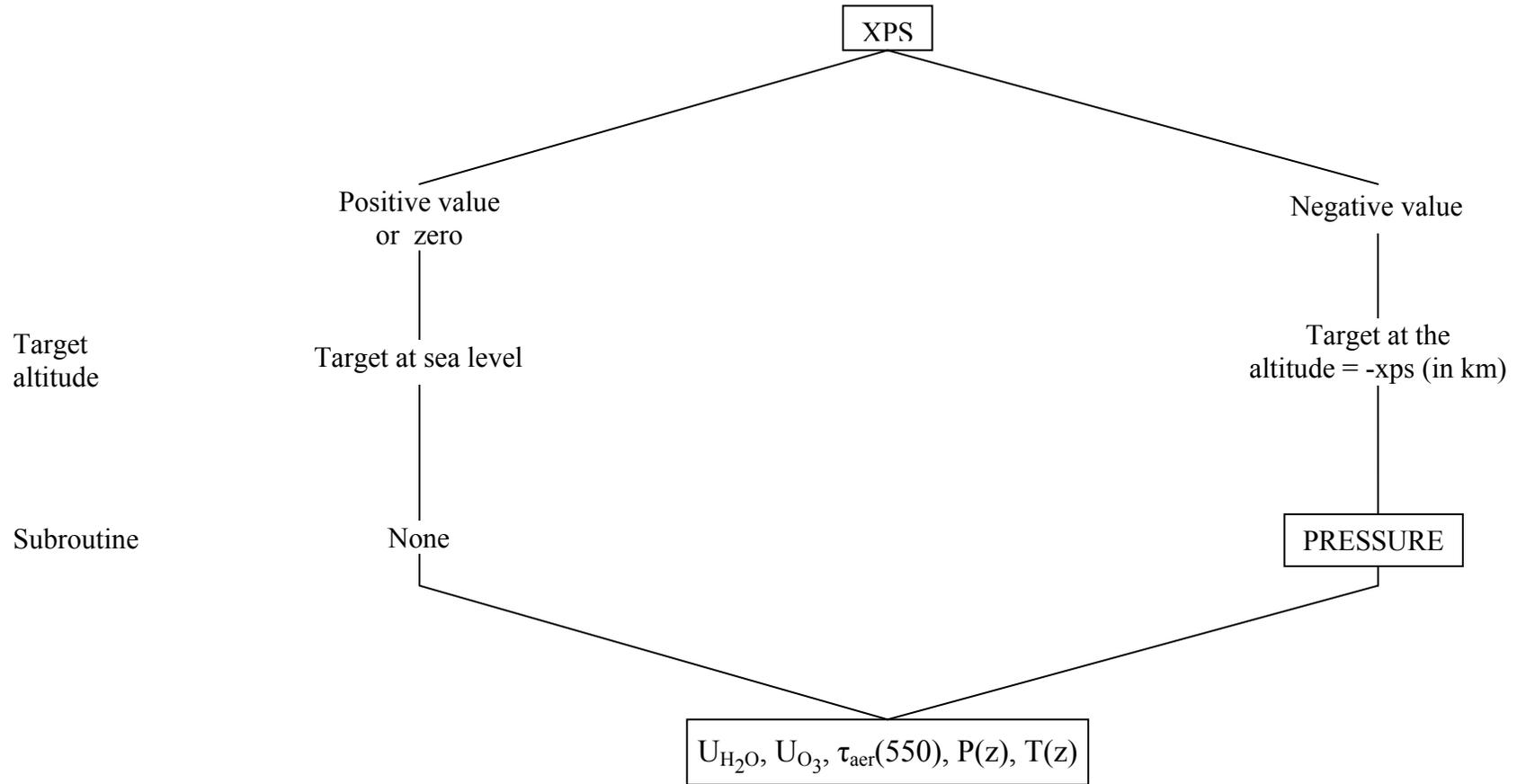
**Fig. A-6.** Detailed flow chart for the effect of altitude: Target.
