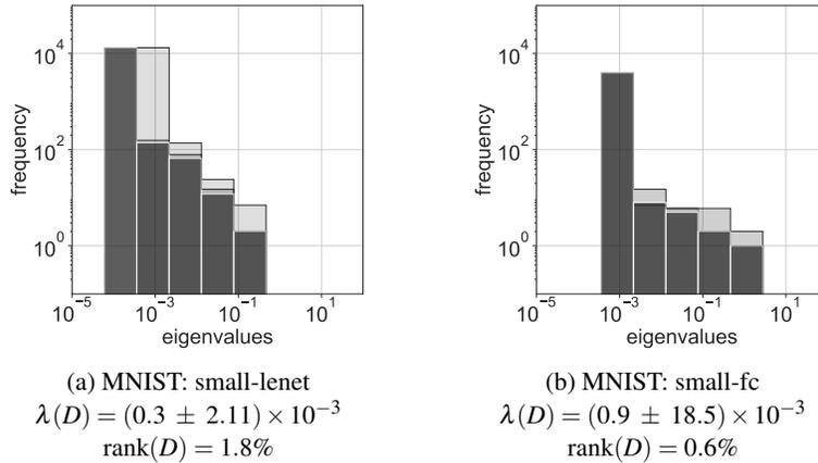
Figure 1: Eigenspectrum of  $D(x)$  at three instants during training (20%, 40% and 100% completion, darker is later). The eigenspectrum in Fig. 1b for the fully-connected network has a much smaller rank and much larger variance than the one in Fig. 1a which also performs better on MNIST. This indicates that convolutional networks are better conditioned than fully-connected networks in terms of  $D(x)$ .
