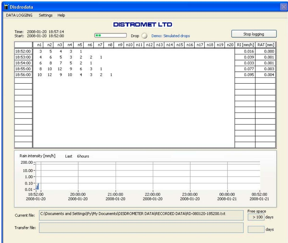
After the START button has been pushed (according to 2.3.4) wait until the indicated start time has been reached and the data logging process starts. (green progress bar is active, showing the time interval).
