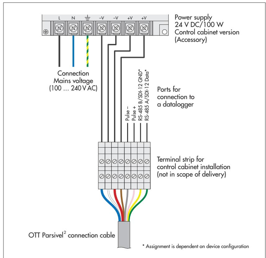
Fig. 18: Connecting power supply protective housing version to the OTT Parsivel<sup>2</sup>.
