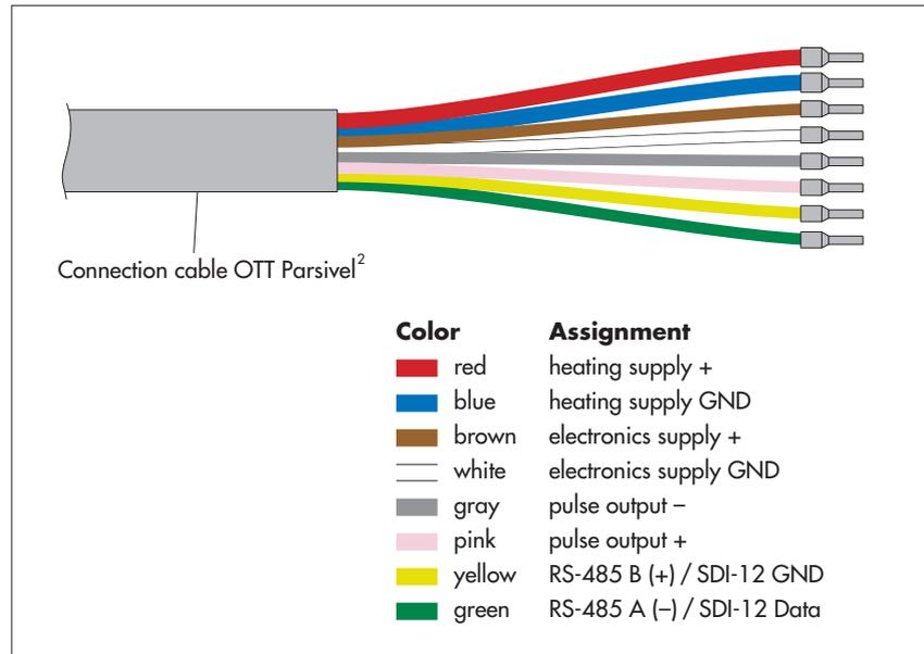
The green and yellow cable is assigned either to the RS-485 or SDI-12 interface. The selection is carried out during setup via the OTT Parsivel user software ASDO or a terminal program. Both of these wires are assigned to the RS-485 interface at the factory.
