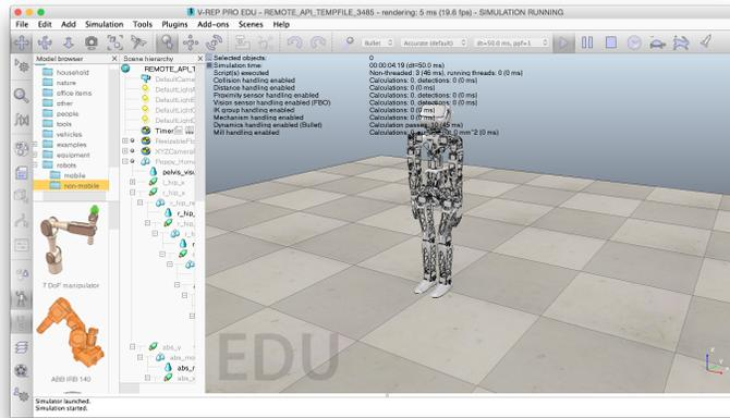
Now you can control the simulated Poppy robot as a real robot, as presented in section 6.
