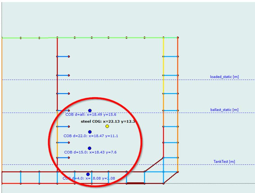
Development of weight and COG is recorded each time the structure changes. The resulting plot can be seen by pressing the “weights” button.
