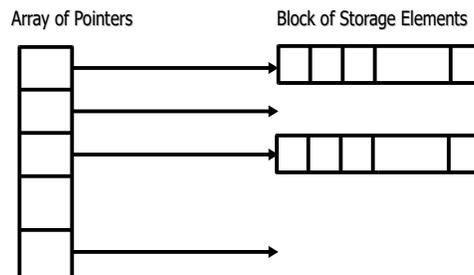
The Array of Pointers is created when the memory is initialized and the size is set. A block of storage is allocated when a write operation writes to a location within the block. This data structure minimizes workstation memory usage when only a portion of the RAM model is used.
