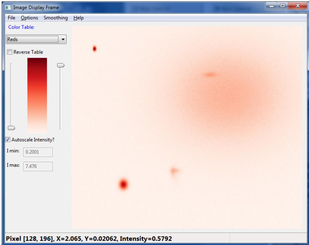
This screenshot shows a long list of choices for color table, a checkbox to reverse the color table, sliders to adjust the upper and lower level, a checkbox to auto-scale the intensity, or entries to set the intensity values for minimum and maximum intensity. Clicking on the image will show its coordinates and intensity value. Click-and-Drag will select a rectangular box to zoom in on a particular feature of the image.
