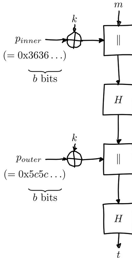
The two pads are XORed with the key before use. The result is either prepended to the original message (for the inner padding  $p_{inner}$ ) or to the intermediate hash output (for the outer padding  $p_{outer}$ ). Because they're prepended, the internal state of the hash function after processing the prefixes can be computed ahead of time, shaving a few cycles off the MAC computation time.
