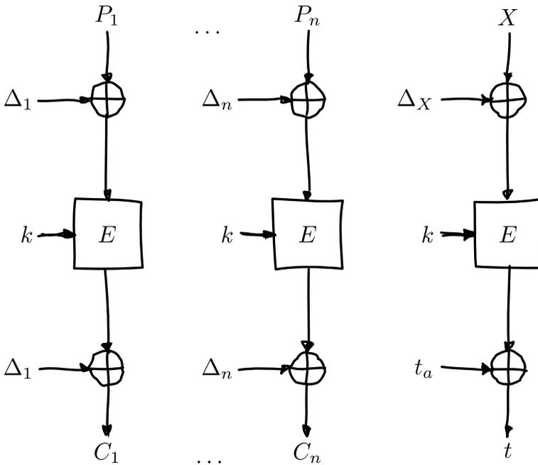
checksum block  $X$  is just all of the plaintext blocks  $P_i$  XORed together. Finally, *OCB mode* is easy to compute in parallel; only the final authentication tag is dependent on all the preceding information.
