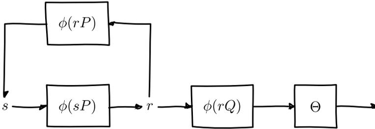
Throughout the algorithm,  $\phi$  is a function that takes a curve point and turns it into an integer. The algorithm needs two given points on the curve:  $P$  and  $Q$ . These are fixed, and defined in the specification. The algorithm has an internal state  $s$ . When producing a new block of bits, the algorithm turns  $s$  into a different value  $r$  using the  $\phi$  function and elliptic curve scalar multiplication with  $P$ :
