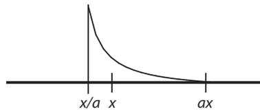
New values are picked from the equivalent of a sliding window on the log-transformed  $x$  axis.
