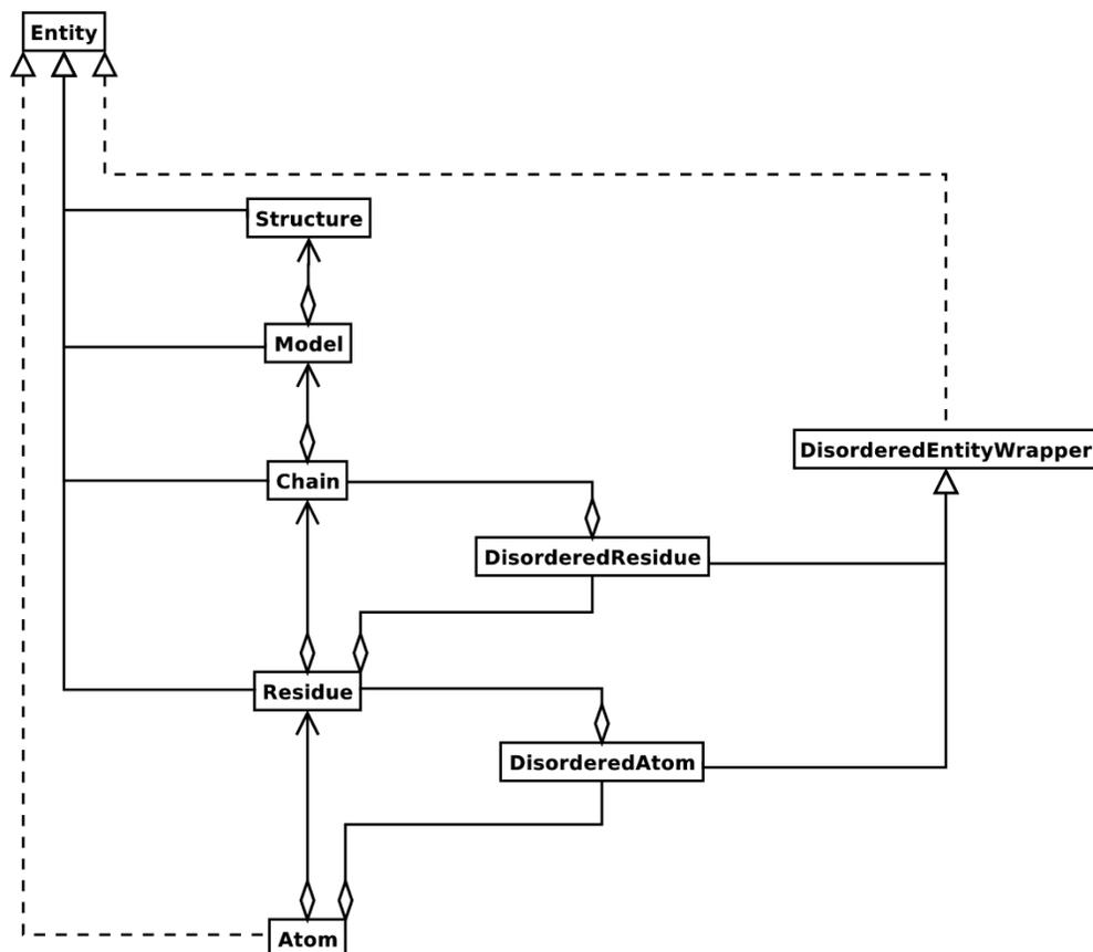
Figure 11.1: UML diagram of SMCRA architecture of the **Structure** class used to represent a macromolecular structure. Full lines with diamonds denote aggregation, full lines with arrows denote referencing, full lines with triangles denote inheritance and dashed lines with triangles denote interface realization.
