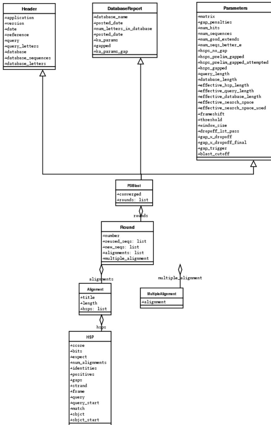
Figure 7.2: Class diagram for the PSIBlast Record class.
