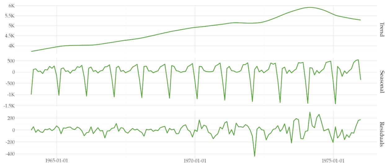
Figure 2: Seasonal, Trend, and Residuals components after decomposition on a monthly frequency using the STL (Season-Trend decomposition using LOESS) method.
