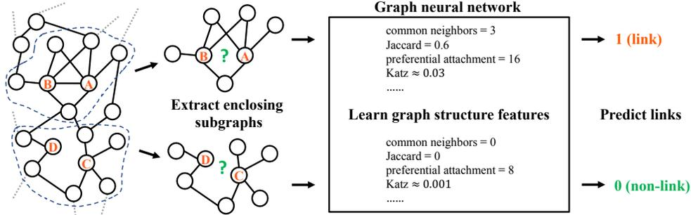
**Figure 1:** The SEAL framework. For each target link, SEAL extracts a local enclosing subgraph around it, and uses a GNN to learn general graph structure features for link prediction. Note that the heuristics listed inside the box are just for illustration – the learned features may be completely different from existing heuristics.
