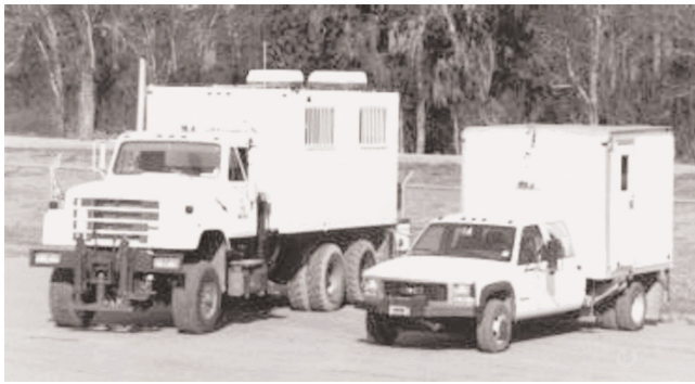
FIGURE 1 Louisiana CPT systems: CIMCPT on the right and REVEGITS on the left.
