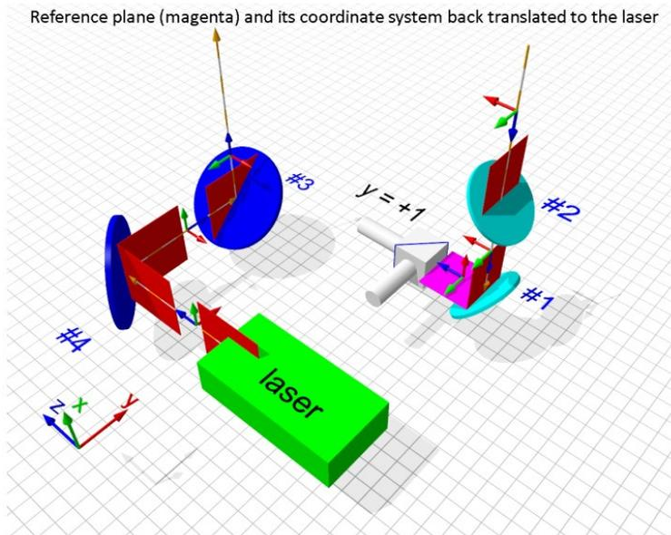
We define  $\gamma = +1$  as in the picture above! Then the reference plane is the incidence plane of the PBC (magenta). The red planes are the back-translations of the reference plane to the incidence and exidence planes of the optical elements. The multiplication of Müller matrices is in direction of the propagation of light.
